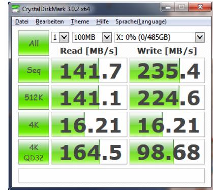
**Test 3. Async vs sync write depending on ZIL, Pool build from 5 x vdevs, each from a basic Seagate 15k/m disks (Raid-0)**
