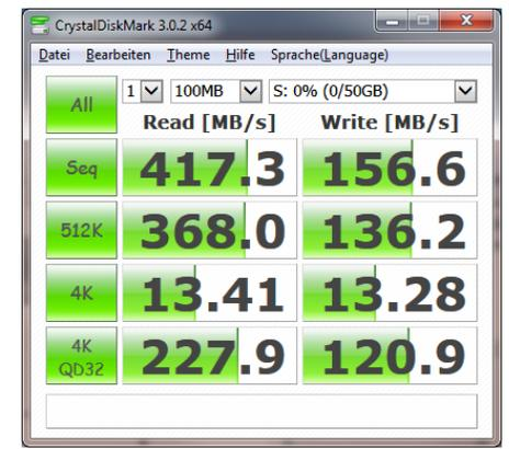
Result for SSD only pool: No need for mirrors, Raid-Z vdevs are ok, a dedicated very fast ZIL is recommended.
